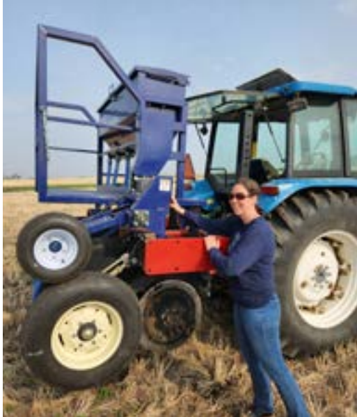
Maryse Bourgault adjusting the rate on custom-made deep fertilizer bander.
